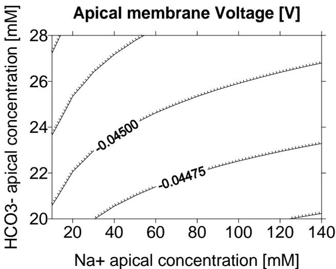
Fig. 4 The potential between cell interior and apical side as a function of concentrations of  $\text{Na}^+$  and  $\text{HCO}_3^-$  ions at apical side. Concentrations of  $\text{K}^+$ ,  $\text{Cl}^-$  remains constant and equal  $X_{\text{K}^+, \text{ap}}=10 \text{ mM}$ ,  $X_{\text{Cl}^-, \text{ap}}=100 \text{ mM}$ .
