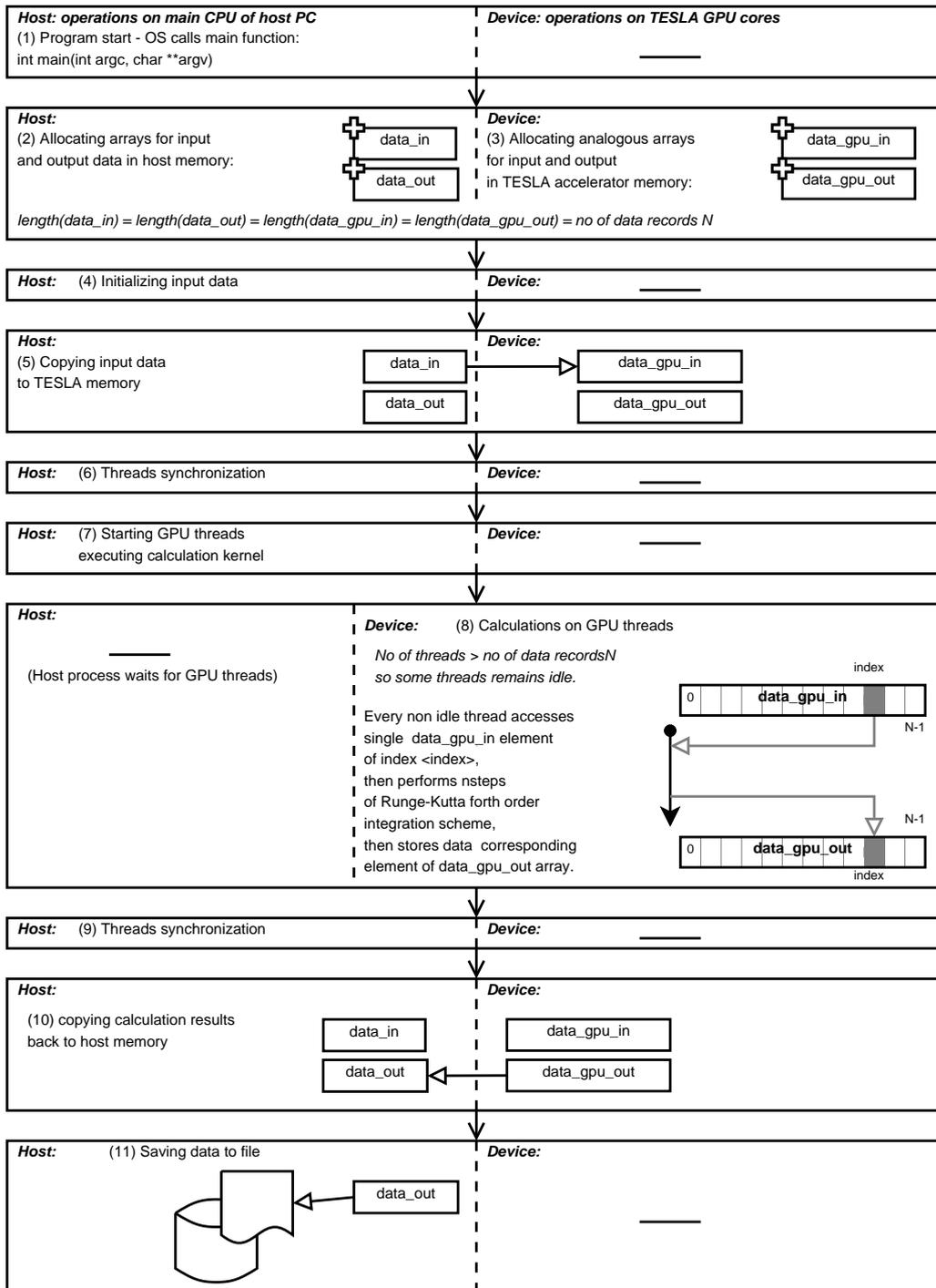
Fig. 2 GPU optimization of multiple identical scalar calculations for different initial data. The most important numerations are numbered. The same enumeration is used in source code comments. The host process reads initial data and parameters, distributes these values in the GPU device memory, and launches appropriate number of GPU device threads. Each GPU thread performs simulation for a single initial data set.
