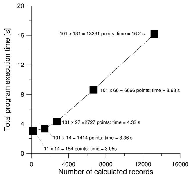
Fig. 10 Tests of scalability of calculations on the TESLA C1060 accelerator with double precision
