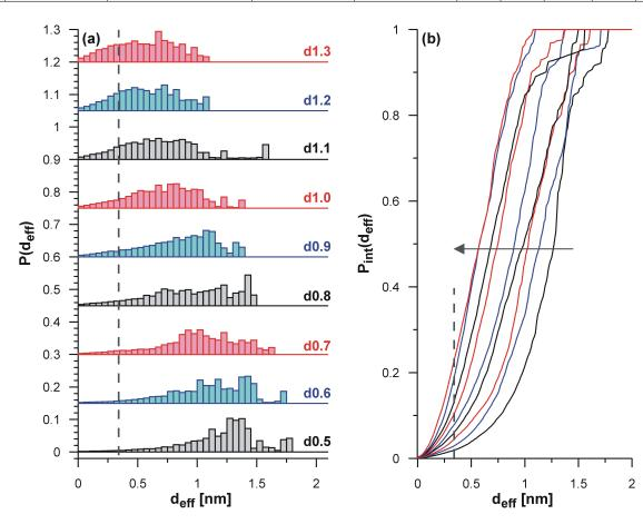
Fig. 3 (a) Histograms of pore diameters for the considered VPCs obtained from BG method (the dashed line represents the size of Ar atoms, subsequent histograms were shifted by 0.15 from the previous ones). (b) Integral curves related to the histograms (the arrow shows the direction of changes from the d0.5 structure up to the d1.3 one).
