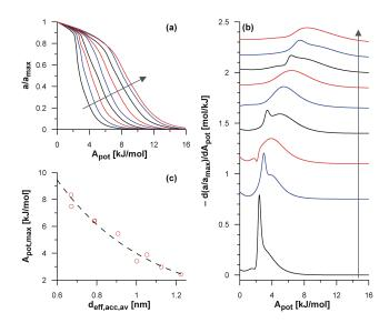
Fig. 6 (a) Characteristic curves connected with isotherms presented in figure 4 (the arrow shows the direction of changes from the d0.5 structure up to the d1.3 one), (b) comparison of APDs for all the considered systems (subsequent curves were shifted by: 0.0, 0.75, 1.1, 1.4, 1.65, 1.85, 2.0, 2.15 and 2.3, respectively) (c) correlation between the location of maximum on APD curve and the average diameter of pores (the dashed line was drawn to guide the eye).
